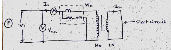
Here sated current of High voltage winding is applied to the primary. Due to current in Primary (II) induces a Current in secondary In
