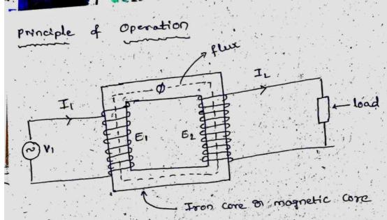
fig: Connection type of transformer
