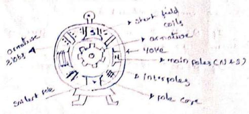
Yoke -> known as magnetic frame. -> stationary part of machine, which produces a regressic April Same feur from main poles. Constraint to > Acts as 2 purposes O to cour the corde mochine 1 Provide the mechanical support
