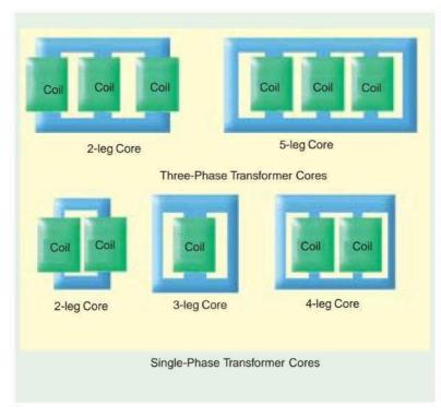
constructing a single 3-phase transformer as shown in Fig. 33.3. It does not differ from three single-phase transformers put side by side. Saving in iron is due to the joint use of the magnetic paths between the coils. The three phases, in this case, are more independent than they are in the core type transformers, because each phase has a magnetic circuit independent of the other.
