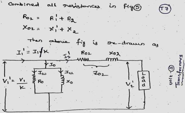
fig@ all parameters separred to secondary
