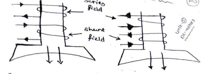
field windings. It series field aids the short field excitation then it is cummulative then it is cummulative then it is cummulative then it is cummulative then it is called opposes the shout field then it is called differentially.
