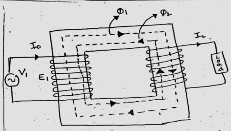
fig stows transformer under load condition
