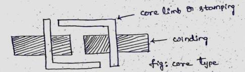
A part of core is sourrounding by the windings.
