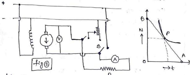
let AB > indicate target to rormal speed  $\frac{dN}{dt} = \frac{OB \text{ in spm}}{OA \text{ in sec}}$
