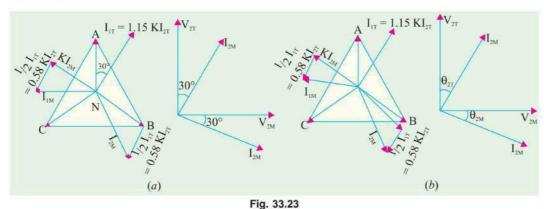
Fig. 33.23 (a) illustrates the condition corresponding to a balanced two-phase load at a lagging power factor of 0.866. The construction is the same as in Fig. 33.22. It will be seen that the 3-phase side is again balanced. But under these conditions, the main transformer rating is 15% greater than that of the teaser, because its voltage is 15% greater although its current is the same.
