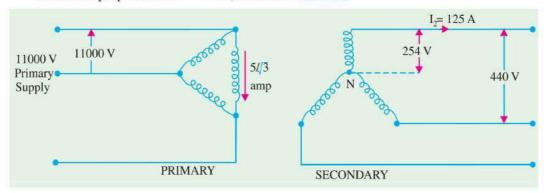
Fig. 33.10. Transformer coil currents
