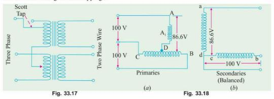
If, in the secondaries of Fig. 33.14 (b), points c and d are connected as shown in Fig. 33.18 (b), then a 2-phase, 3-wire system is obtained. The voltage  $E_{dc}$  is 86.6 V but  $E_{Cb} = 100$  V, hence the
