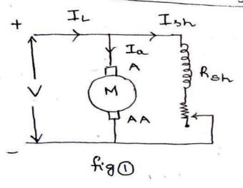
In this Connection, field winding is Connecte across the armature of the rooter.
