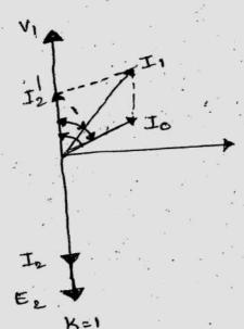
fig@ phasor diagrams for non inductive load (Resistive Load)
